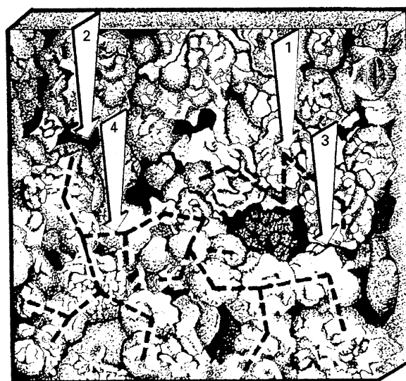
Figure 11 Sketch of the aggregate-to-aggregate conduction in a polyester medium. (1) Aggregates of nickel covered with insulating polyester film, (2) insulating medium, (3) interstitial spaces, (4) conducting paths.
